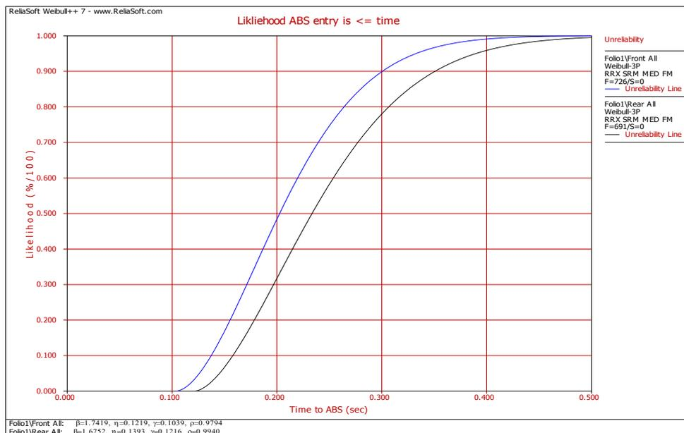
34. By reducing the lower limit to 0.1 seconds the test failure rate reduces to practically zero. Allowing the reduction tends to make the regulation more stringent by including a greater number of brake force application rates and eliminates restrictive test requirements.
