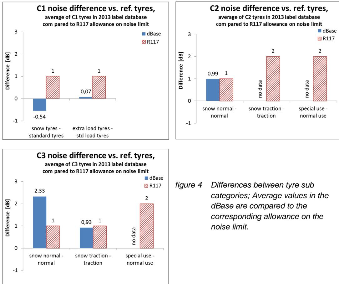
figure 4 Differences between tyre sub categories; Average values in the dBase are compared to the corresponding allowance on the noise limit.
