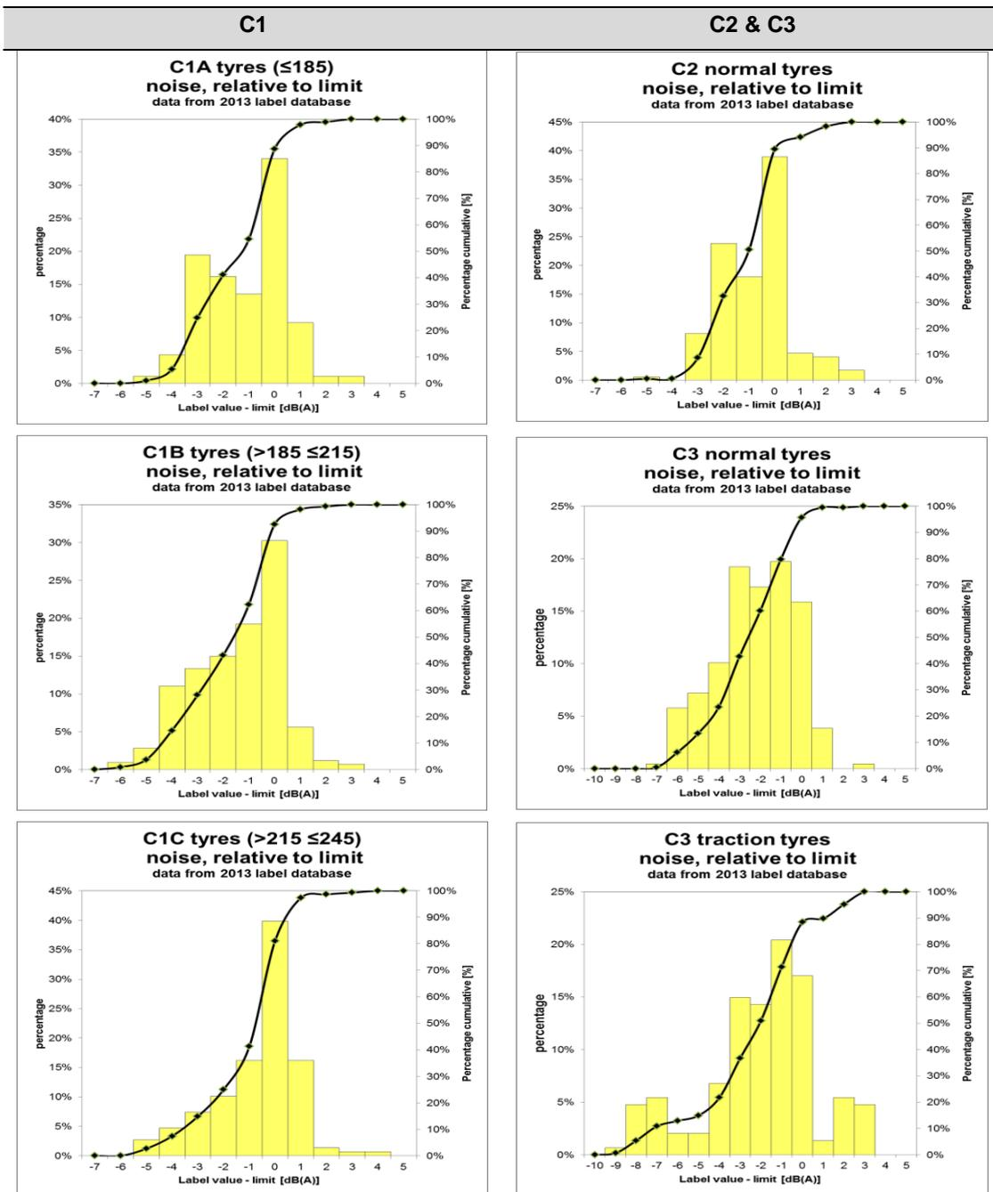
figure 3 Statistical distribution of tyre noise dB emission values relative to the limit. The limits may consist of the sum of the base limit plus a margin for special properties (snow use etc) if relevant.
