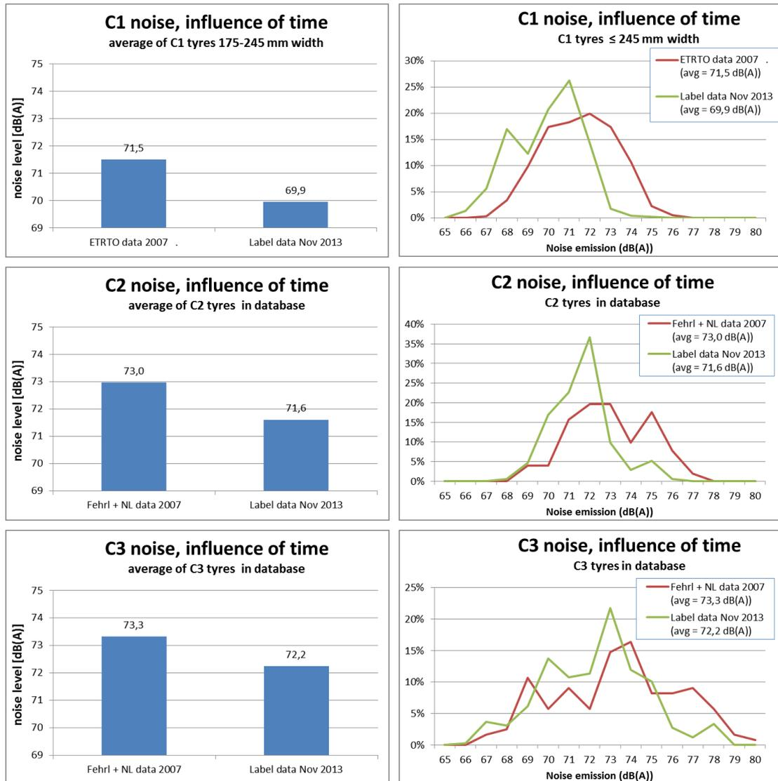
figure 2 Tyre noise data of 2013 compared to data of 2007. The left graphs show the effect on the average values. The right graphs show the distribution over noise classes of 1 dB.
