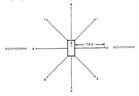
The measurement is performed at the stationary vehicle according to Figure 1, using two microphone positions at a distance of  $7\,\mathrm{m}$  from the contour of the vehicles, and at  $1.2\,\mathrm{m}$  above ground.
