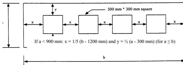
If  $a < 900$  mm:  $x = 1/5 (b - 1200 \text{ mm})$  and  $y = 1/2 (a - 300 \text{ mm})$  (for  $a \leq b$ )
