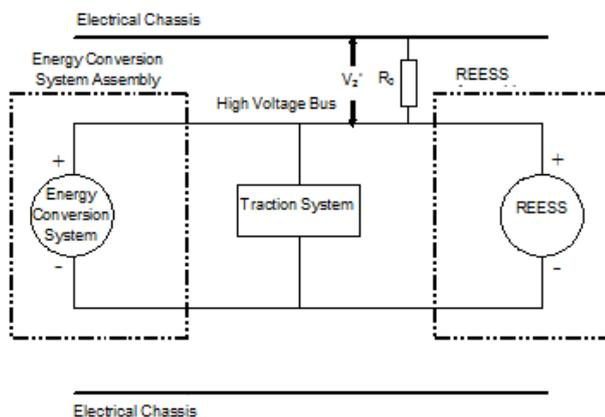
*Note:* The standard known resistance  $R_0$  (in  $\Omega$ ) should be the value of the minimum required isolation resistance ( $\Omega/V$ ) multiplied by the working voltage ( $V$ ) of the vehicle plus/minus 20 per cent.  $R_0$  is not required to be precisely this value since the equations are valid for any  $R_0$ ; however, a  $R_0$  value in this range should provide a good resolution for the voltage measurements.
