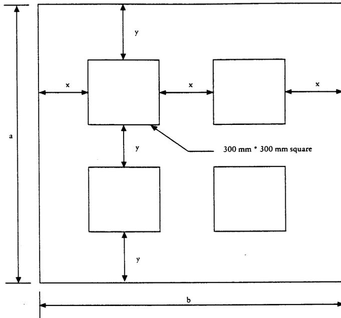
If  $a \geq 900$  mm:  $x = 1/3 (b - 600\text{mm})$  and  $y = 1/3 (a - 600\text{mm})$  (for  $a \leq b$ )
