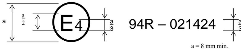
The above approval mark affixed to a vehicle shows that the vehicle type concerned has, with regard to the protection of the occupants in the event of a frontal collision, been approved in the Netherlands (E 4) pursuant to Regulation No. 94 under approval number 021424. The approval number indicates that the approval was granted in accordance with the requirements of Regulation No. 94 as amended by the 02 series of amendments.
