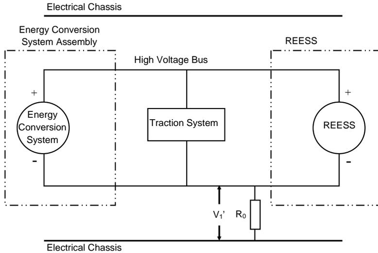
If  $V_2$  is greater than  $V_1$ , insert a standard known resistance ( $R_0$ ) between the positive side of the high voltage bus and the electrical chassis. With  $R_0$  installed, measure the voltage ( $V_2'$ ) between the positive side of the high voltage bus and the electrical chassis (see Figure 4 below).
