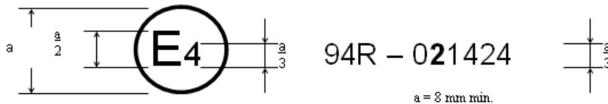
The above approval mark affixed to a vehicle shows that the vehicle type concerned has, with regard to the protection of the occupants in the event of a frontal collision, been approved in the Netherlands (E4) pursuant to Regulation No. 94 under approval number 021424. The approval number indicates that the approval was granted in accordance with the requirements of Regulation No. 94 as amended by the 02 series of amendments.
