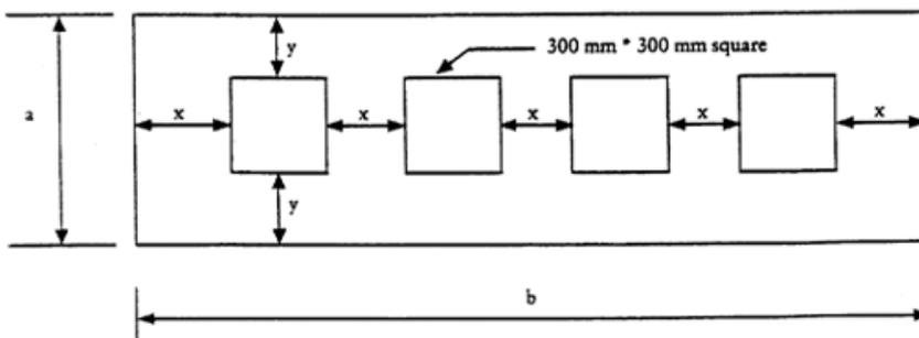
If  $a < 900$  mm:  $x = 1/3 (b - 1\ 200 \text{ mm})$  and  $y = 1/3 (a - 300 \text{ mm})$  (for  $a \leq b$ )
