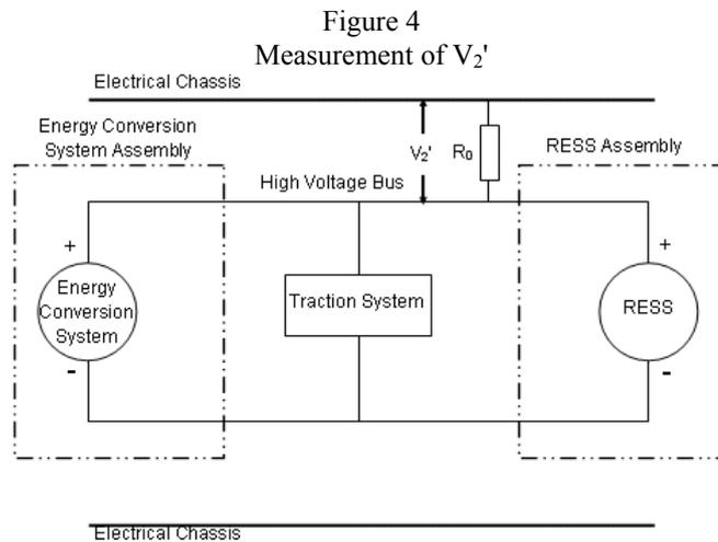
Note 1: The standard known resistance  $R_0$  (in  $\Omega$ ) should be the value of the minimum required isolation resistance ( $\Omega/V$ ) multiplied by the working voltage (V) of the vehicle plus/minus 20 per cent.  $R_0$  is not required to be precisely this value since the equations are valid for any  $R_0$ ; however, a  $R_0$  value in this range should provide a good resolution for the voltage measurements.
