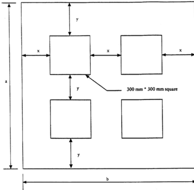
If  $a \geq 900$  mm:  $x = 1/3 (b - 600 \text{ mm})$  and  $y = 1/3(a - 600 \text{ mm})$  (for  $a \leq b$ )
