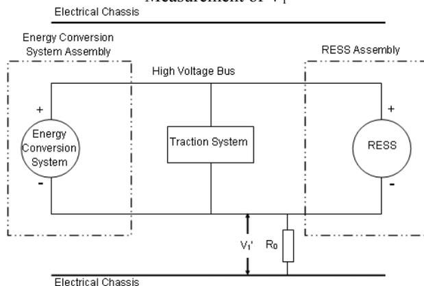
If  $V_2$  is greater than  $V_1$ , insert a standard known resistance ( $R_0$ ) between the positive side of the high voltage bus and the electrical chassis. With  $R_0$  installed, measure the voltage ( $V_2'$ ) between the positive side of the high voltage bus and the electrical chassis (see figure 4).
