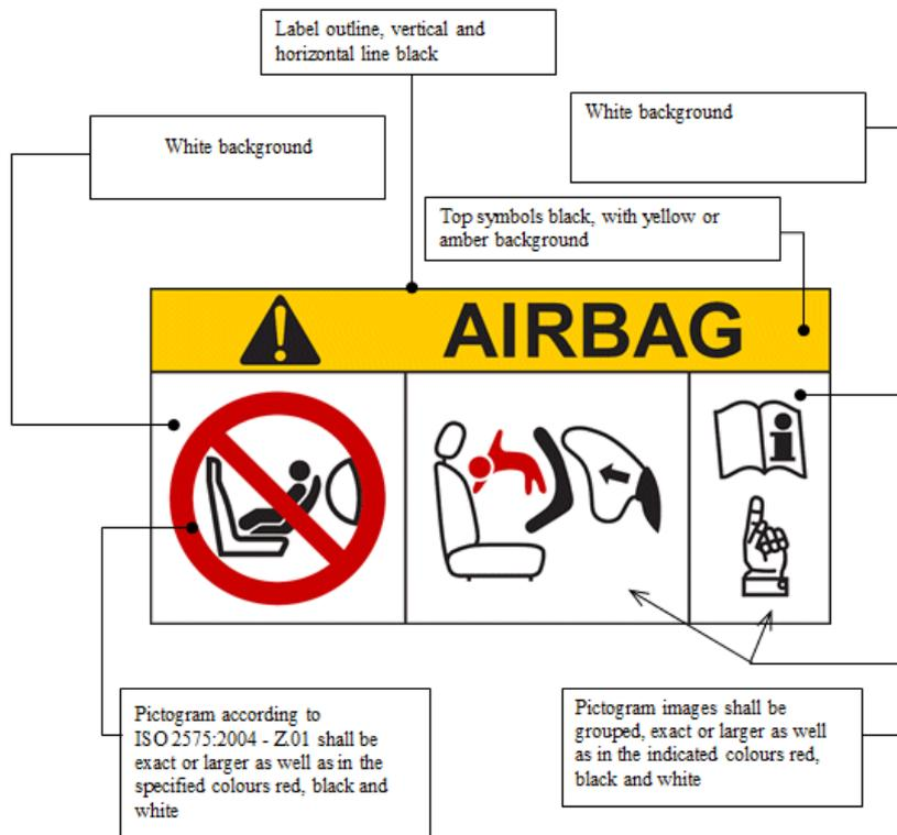
The overall dimensions shall be at least 120 x 60 mm or the equivalent area.
