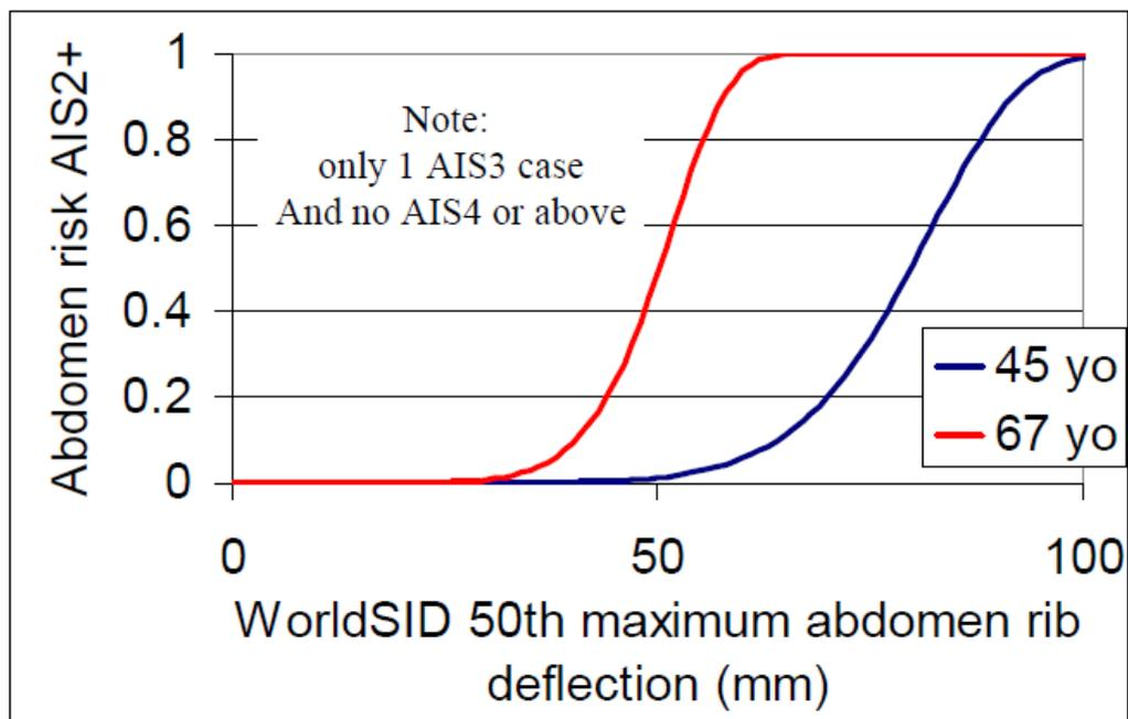
\* Measured by 1D IR-TRACC
