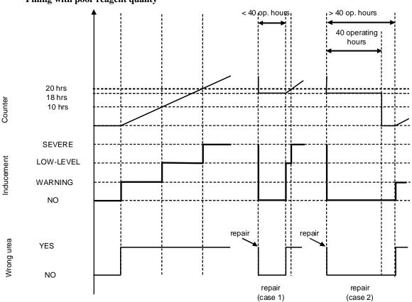
5.4. Figure 7 illustrates three cases of failure of the urea dosing system. This figure also illustrates the process that applies in the case of the monitoring failures described in paragraph 9. of this annex.
