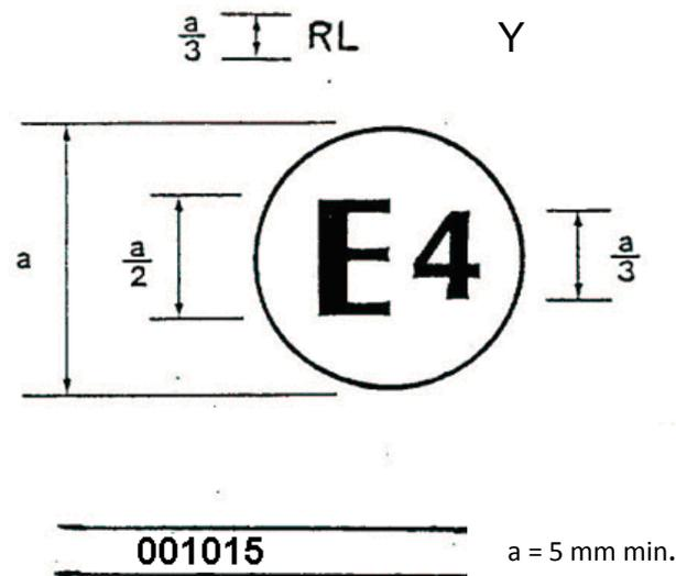
The lamp bearing the approval mark shown above has been approved in the Netherlands (E4) under number 001015 as a part of an interdependent lamp system composing a daytime running lamp. The approval number indicates that the approval was granted according to the requirements of this Regulation in its original (un-amended) form. "
