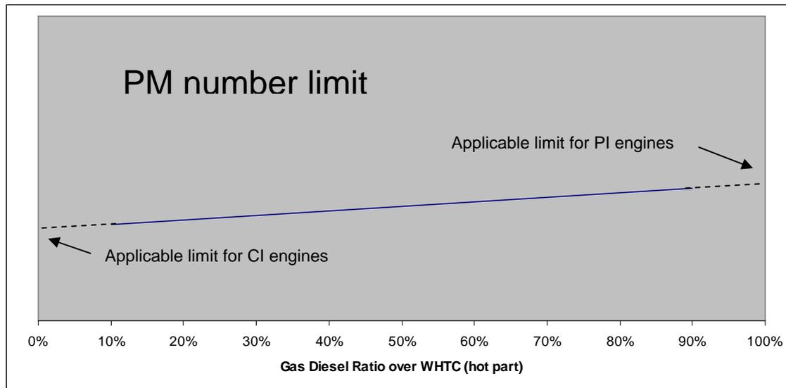
figure 2: illustration of the PN limits in the case of a HDDDF type2 engine operating in dual-fuel mode during the WHTC cycle
