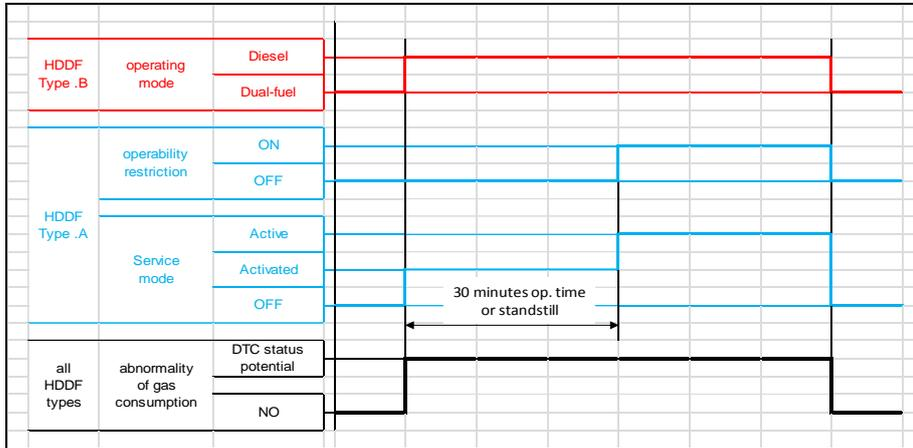
In that use case the service mode is activated (in the case of a Type A HDDF) or the engine switches to Diesel mode (in the case of a Type B HDDF) as soon as the DTC gets the “potential” status (1<sup>st</sup> detection).
