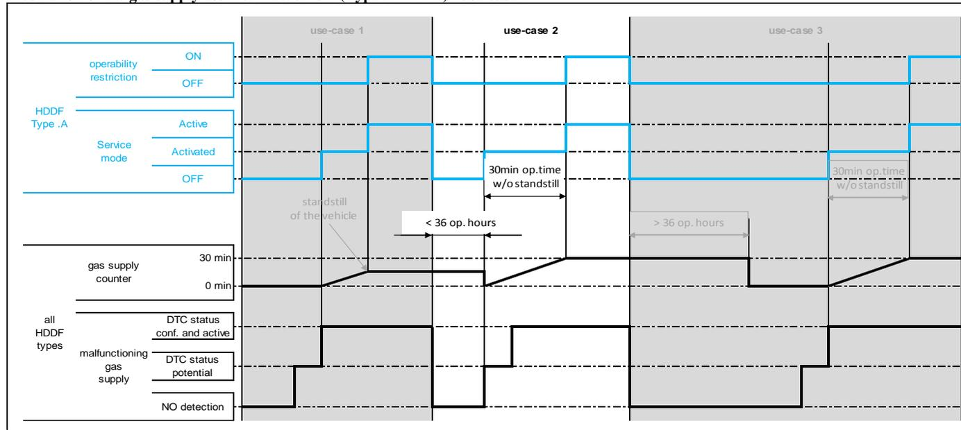
A malfunction of the gas supply is detected while the gas supply malfunction counter is not at zero (in this use-case it indicates the value it reached in use-case 1 when the vehicle became standstill).
