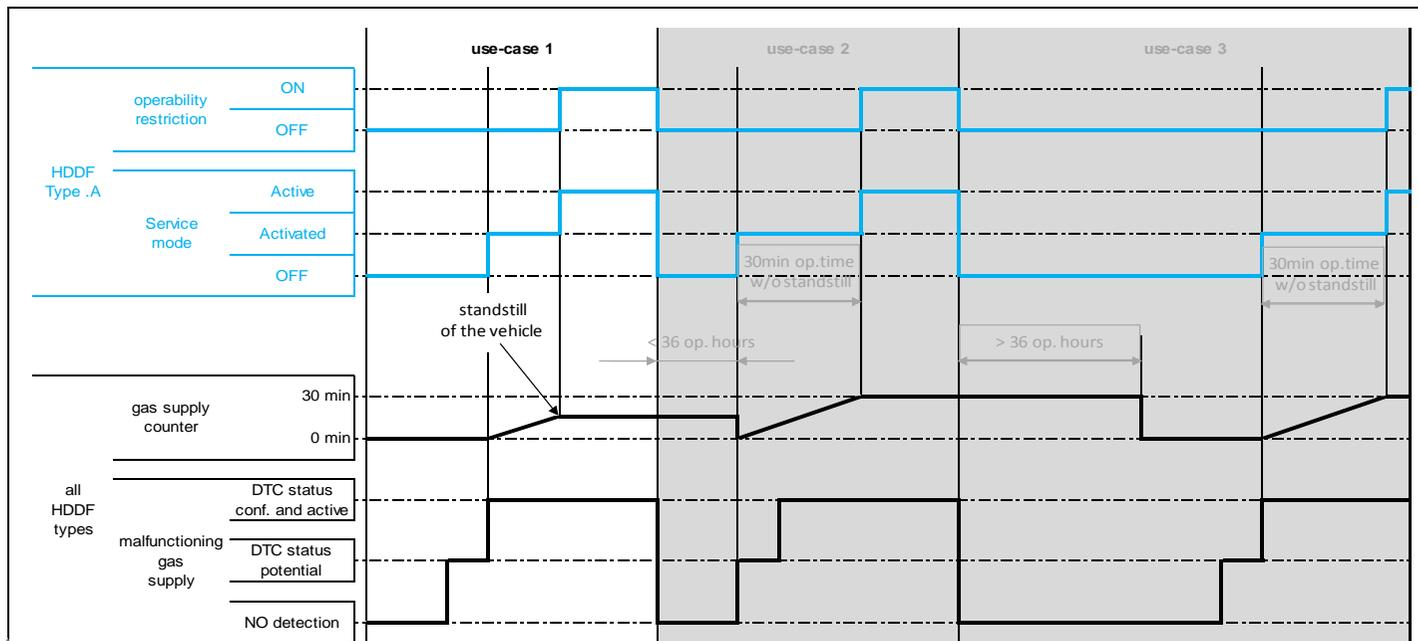
**A malfunction of the gas supply is detected for the very first time.**
