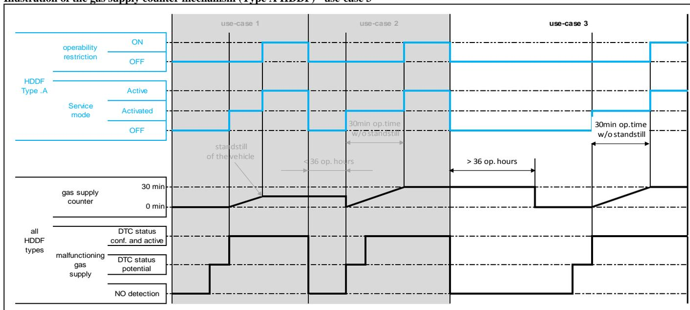
After 36 operating hours without detection of a malfunction of the gas supply, the counter is reset to zero (see paragraph A.2.1.2.3.2.1).
