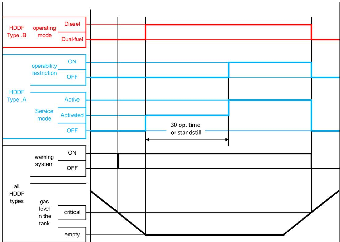
Figure A2.2 – Illustration of the events occurring in case of an empty gas tank (Types A and B Hddf)
