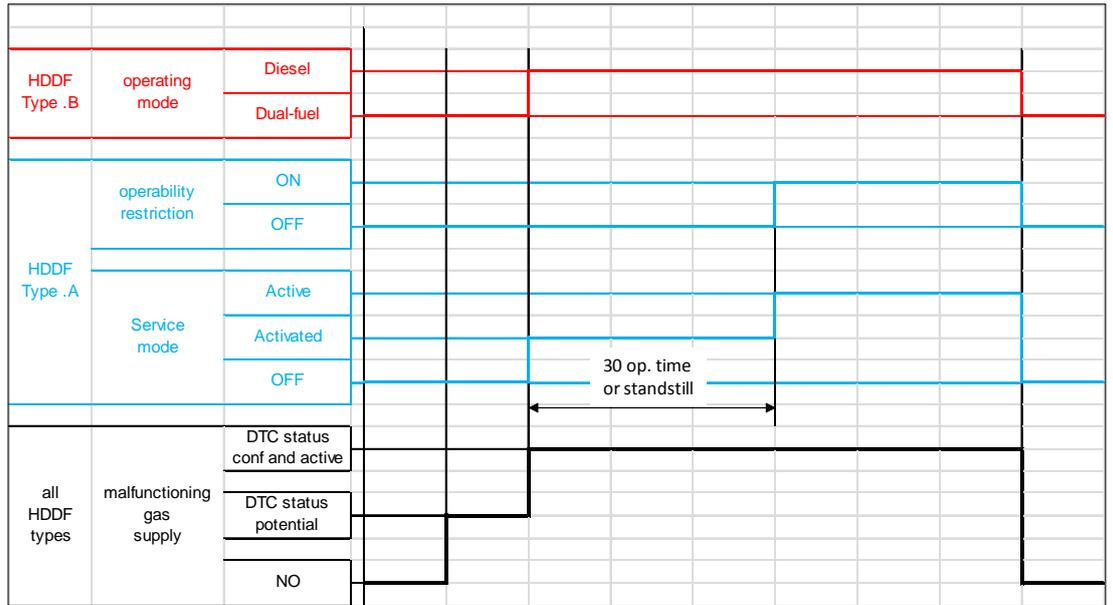
Figure A2.3 – Illustration of the events occurring in case of a malfunctioning gas supply system (Types A and B HDDF)
