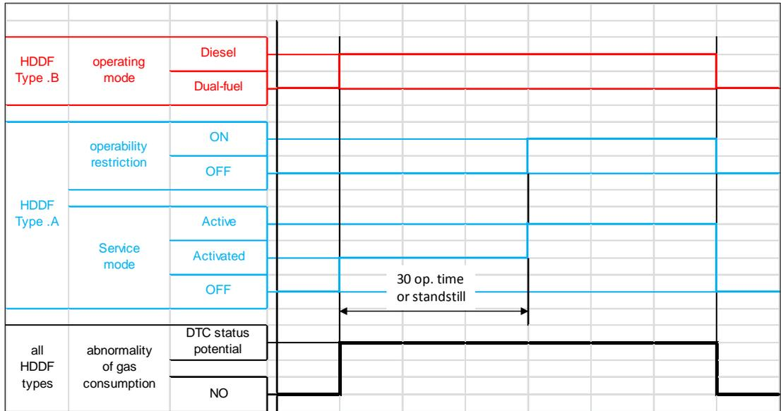
Figure A2.4 – Illustration of the events occurring in case of abnormality of gas consumption (Types A and B HDDF)
