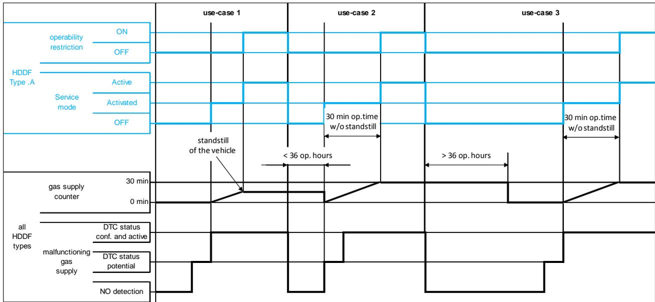
Figure A2.1 – Illustration of the gas supply counter mechanism (Type A HDDF - 3 use-cases)
