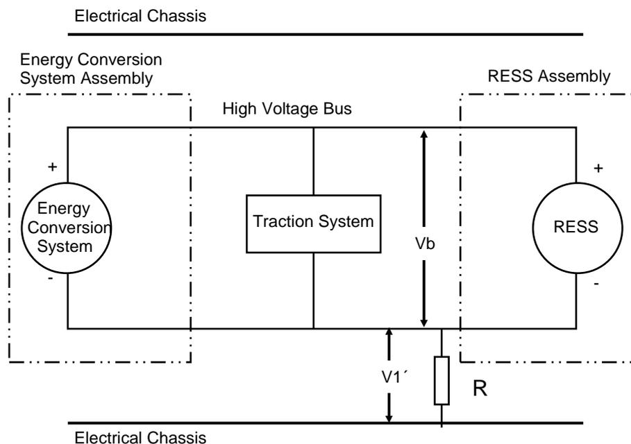
If V2 is greater than V1, insert a standard known resistance (Ro) between the positive side of the high voltage bus and the electrical chassis. With Ro installed, measure the voltage (V2') between the positive side of the high voltage bus and the electrical chassis. (See Figure 3). Calculate the electrical isolation (Ri) according to the formula
