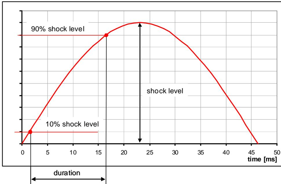
~~The test pulse shall describe a half sinus with duration of 15ms between 10% and 90% of the shock level.~~
