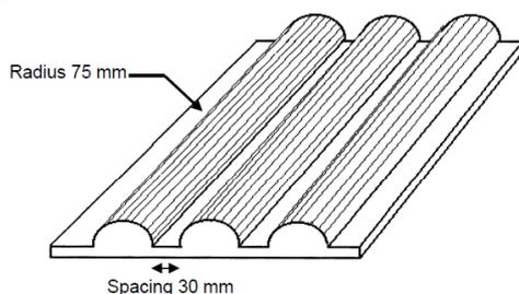
[Dimension of the crush plate:
