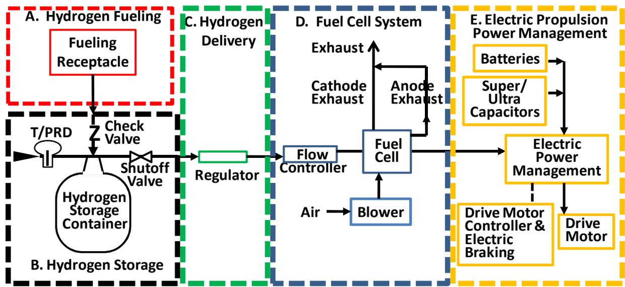
Figure A.1. Example of High-level Schematic of Key Systems in HFCVs
