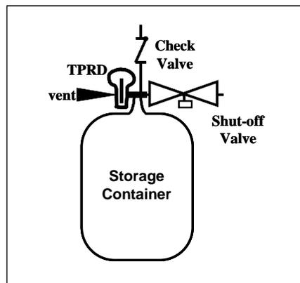
**Figure A.3. Typical Compressed Hydrogen Storage System**
