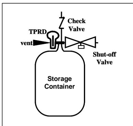
Figure B.5.1.1 Typical Compressed Hydrogen Storage System
