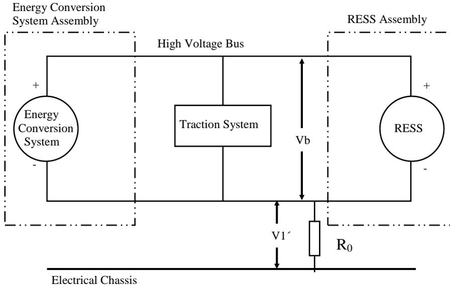
**Figure 2: Measurement of V1'**
