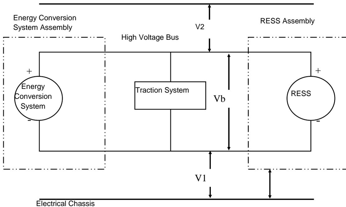
**Figure 1 Measurement of Vb, V1, V2**
