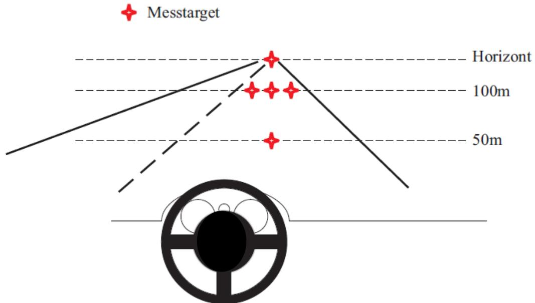
Figure 5: Positions of the test targets for the evaluation of the adaptation level.
