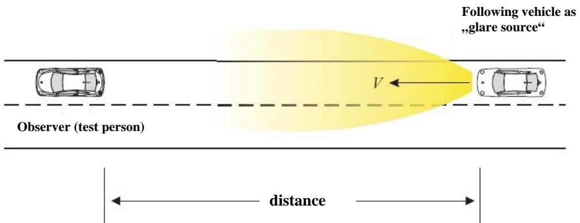
Figure 4: Experimental design of the second part of the experiment.
