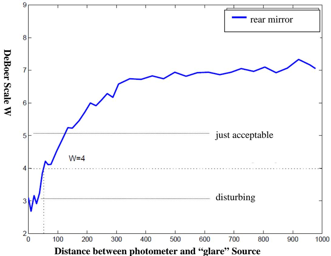
Figure 3: Calculated DeBoer levels, W, according to the relationship of Bindel and Schmidt-Clausen <sup>2/</sup> on the basis of the photometric measurements.
