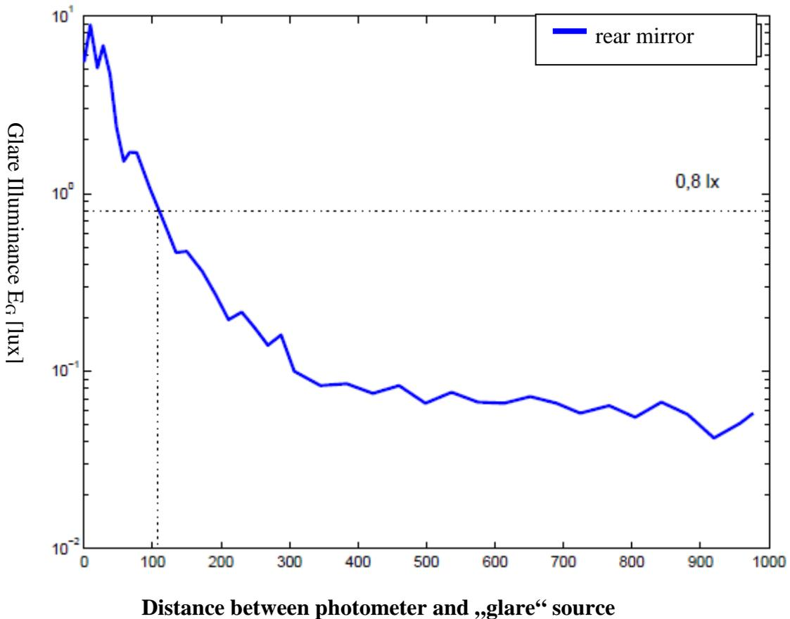
Figure 2: Measured values in relation to the distance between photometer and "glare" source
