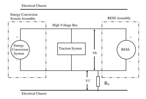
If V2 is greater than V1, insert a standard known resistance (Ro) between the positive side of the high voltage bus and the electrical chassis. With Ro installed, measure the voltage (V2') between the positive side of the high voltage bus and the electrical chassis. (See Figure 3). Calculate the electrical isolation (Ri) according to the formula shown. Divide this electrical isolation value (in  $\Omega$ ) by the nominal operating voltage of the high voltage bus (in volts).
