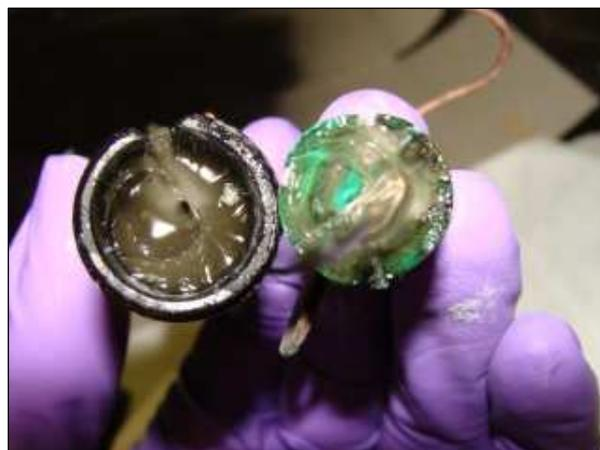
**Figure 4: Residue left in a test cell after a 'Go' (left) and 'No-go' (right) event.**
