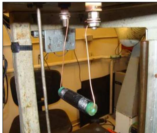
Figure 2: Open 4-L pressure vessel with suspended test cell and instrumentation (left) and close-up of a test cell suspended by copper leg wires connected to electrodes (right).
