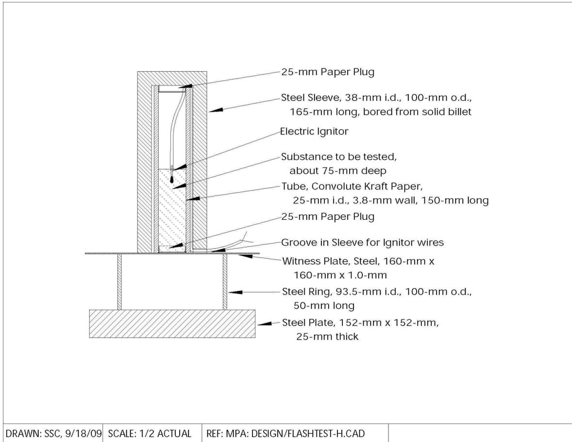
**Figure 2 – DDT Test Apparatus for flash compositions photographs**
