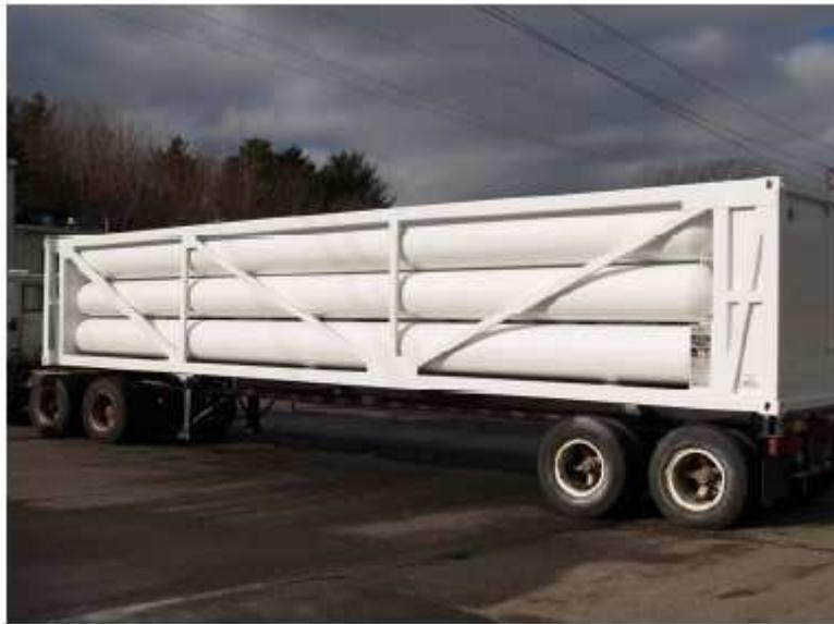
Figure 1: 40-foot-long MEGC (full-length and full-height – 12 tubes)
