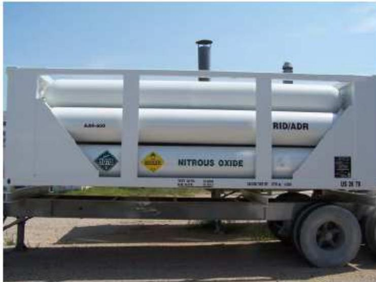
Figure 4: 20-foot-long MEGC (half-length and full-height – 10 tubes)
