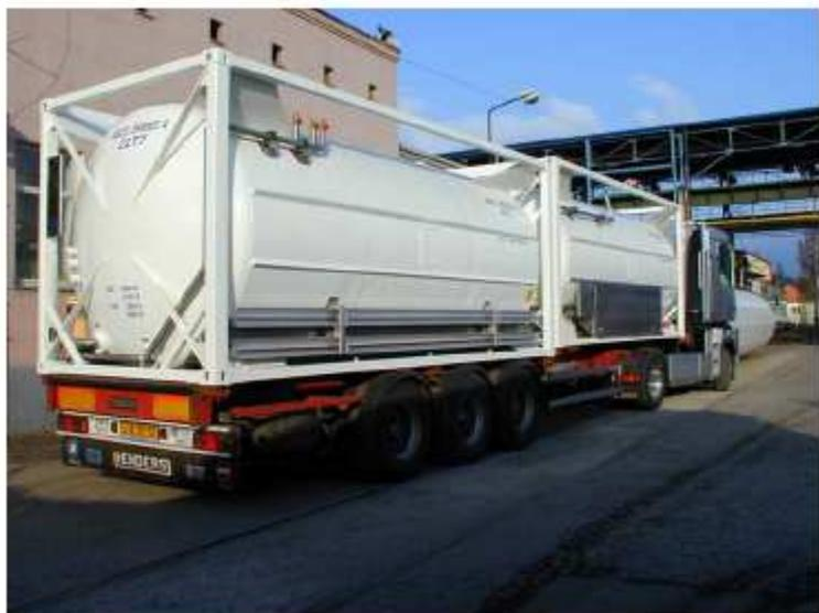
Figure 10: Vacuum-jacketed cryogenic portable tank
