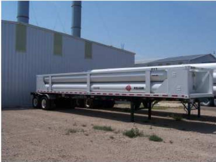
Figure 3: 40-foot-long MEGC (full-length and half-height – 8 tubes)
