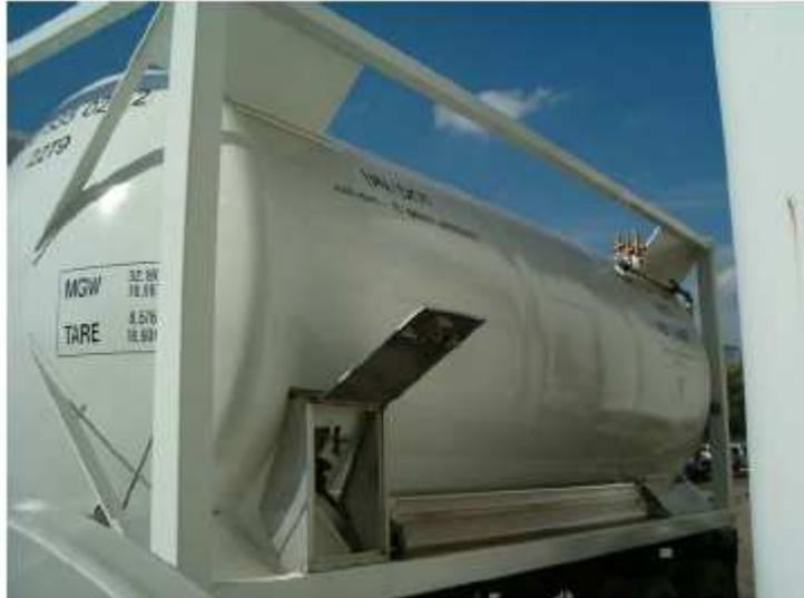
Figure 11: Vacuum-jacketed cryogenic portable tank
