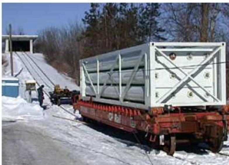
Figure 2: MEGC undergoing an impact test
