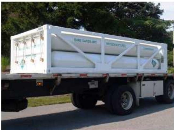
Figure 6: 20-foot-long MEGC (half-length and half-height – 8 tubes)
