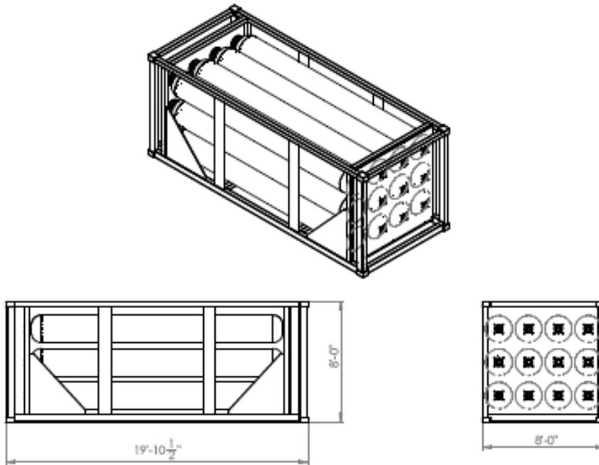
Figure 5: Drawing of 20-foot MEGC (half-length and full-height – 12 tubes)
