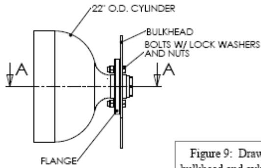
Figure 9: Drawing of MEGC bulkhead and cylinder attachment
