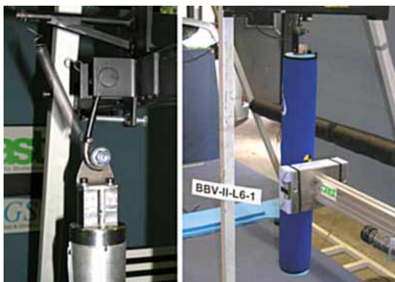
Figure 2. Support system for the legform with release spring (left) and position of impactor relative to point of impact (right).
