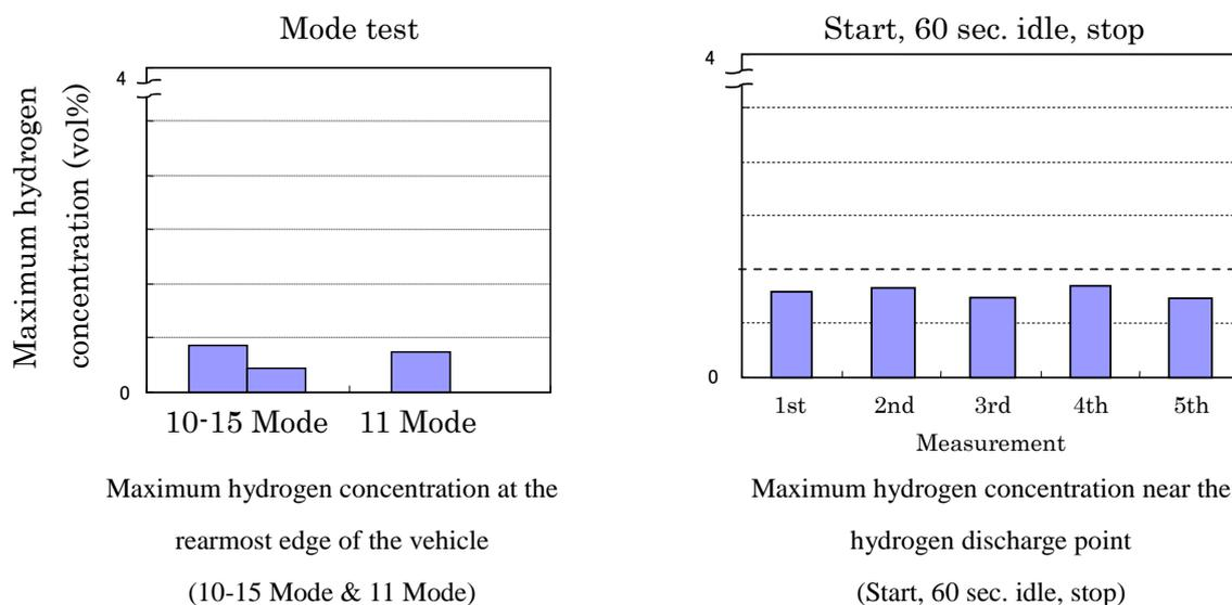
Figure 3 Results of Tests to Check Hydrogen Concentration in Discharged Gas
