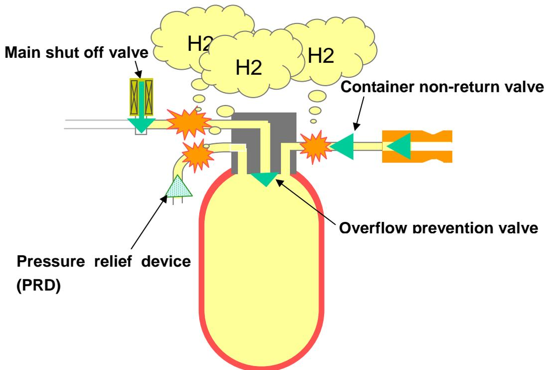
Without the installation requirement to “install the main shut off valve, PRD, and container non-return valve directly on the container”
