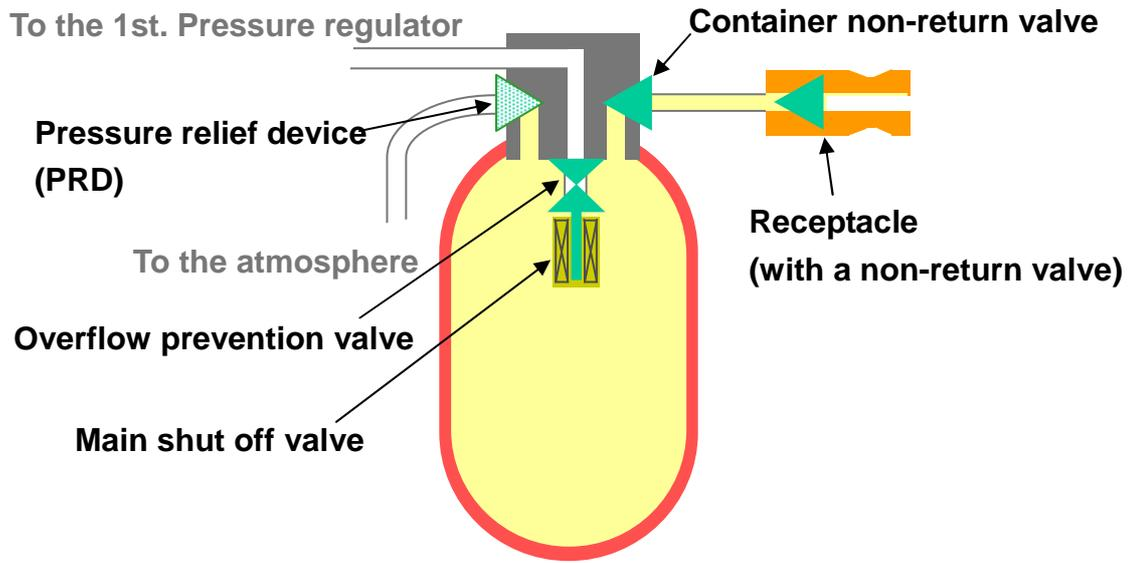
With the installation requirement to “install the main shut off valve, PRD, and container non-return valve directly on the container”
