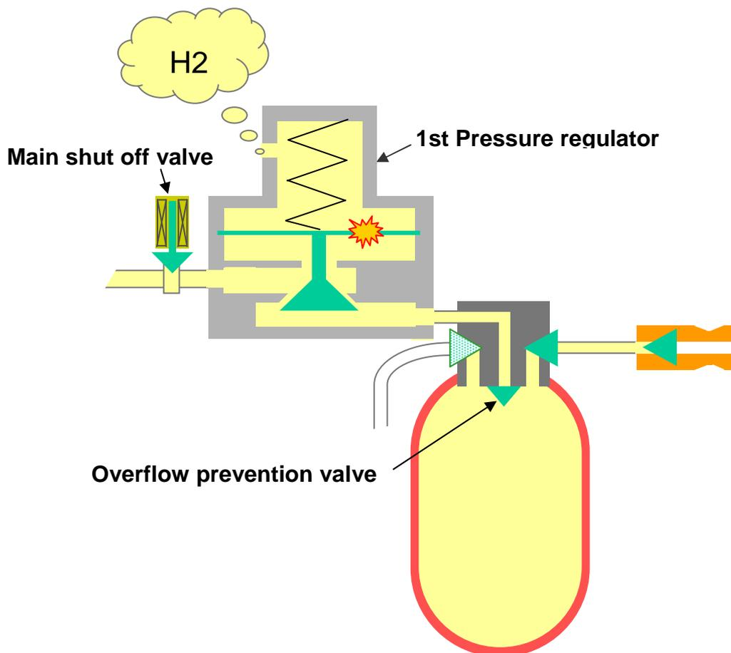
Figure 2 Prohibition to Install the First Pressure Regulator Upstream of the Main Shut Off Valve
