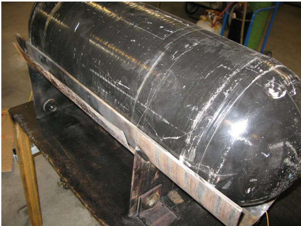
Figure 5 – Note annular space between cradle and shielding for exhaust gases.
