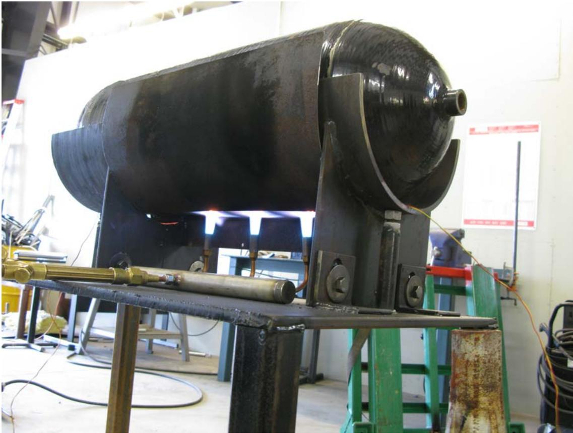
Figure 3 – Torches heating underside of steel cradle.
