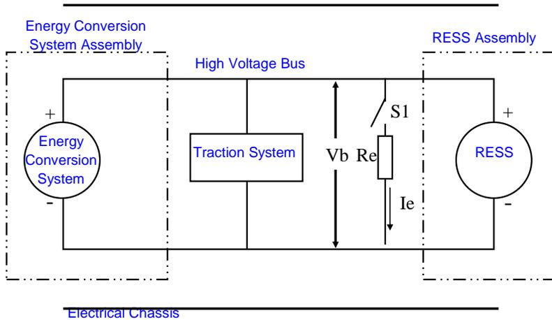
Figure 4: Measurement of high voltage bus energy
