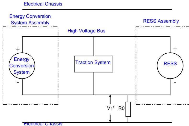
Figure 2: Measurement of V1'
