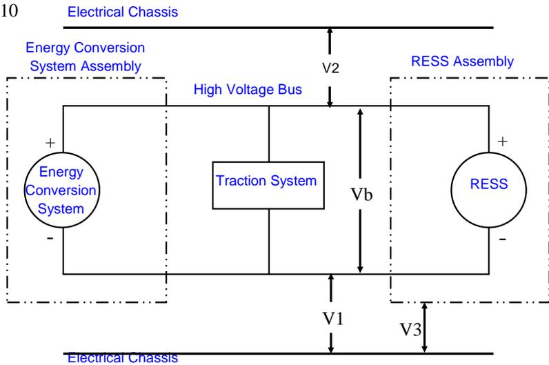
Figure 1: Measurement of  $V_b$ ,  $V_1$ ,  $V_2$
