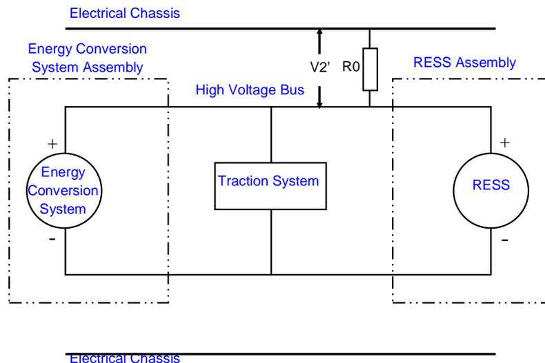
Figure 3: Measurement of V2'
