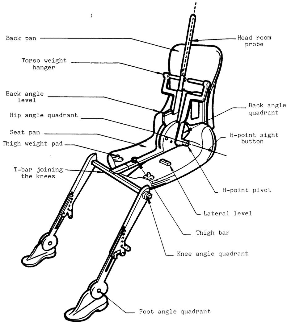
Figure 1 - 3-D H machine element designation
