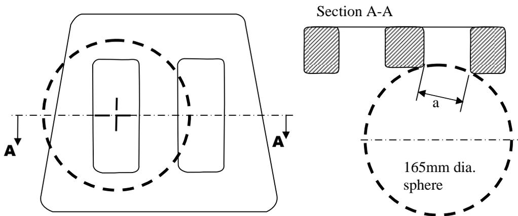
Figure 3-2 - Measurement of a vertical gap "a".
