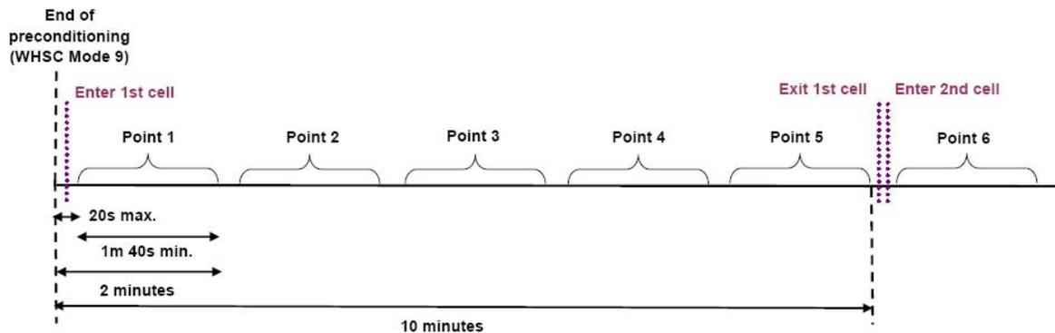
Figure 4: Schematic example of the start of the WNTTE test cycle
