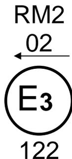
The device bearing the approval mark shown above is a rear end-outline marker lamp with variable luminous intensity approved in Italy (E3) under approval number 122 pursuant to Regulation No. 7.
