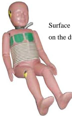
Surface pressure gauge installed on the dummy's abdomen
