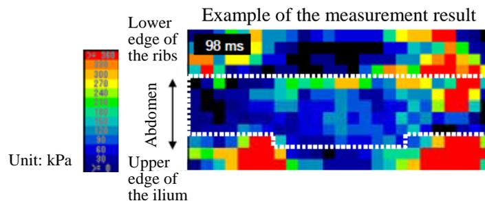
In the past measurements on seven impact-shield type CRSs using the surface pressure gauge, large chest deflections and bottoming-out of the ribs on the thoracic spine were observed in all the tested CRSs and large abdominal loads in some of these CRSs.
