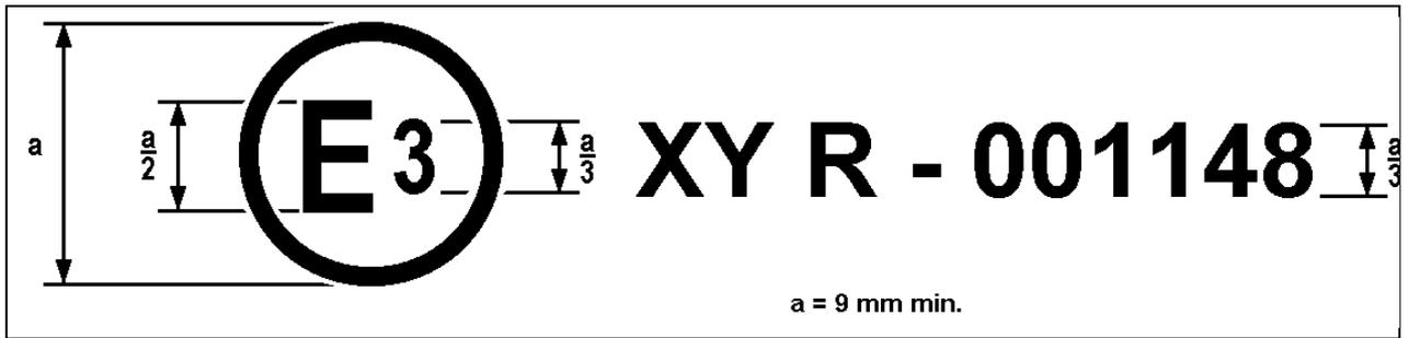
The TBW or TLAS or TPMS bearing the above approval mark is a TBW or TLAS or TPMS that has been approved in Italy (E3) under approval number 001148.
