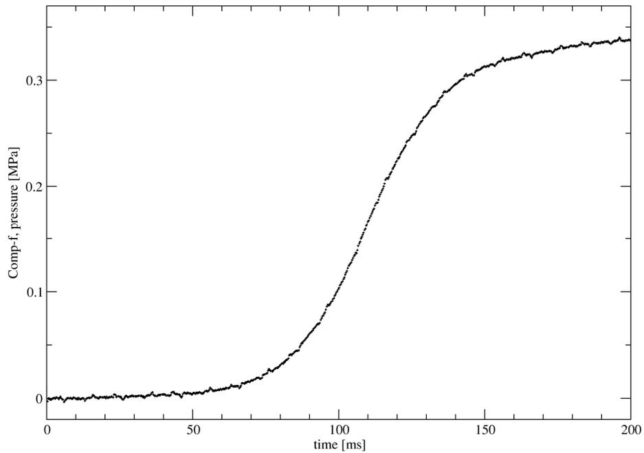
**comp-f:** Analysis of rise-time  $t_{UN2c}$  is not possible since pressures were not achieved. More substance may be required in the test volume.
