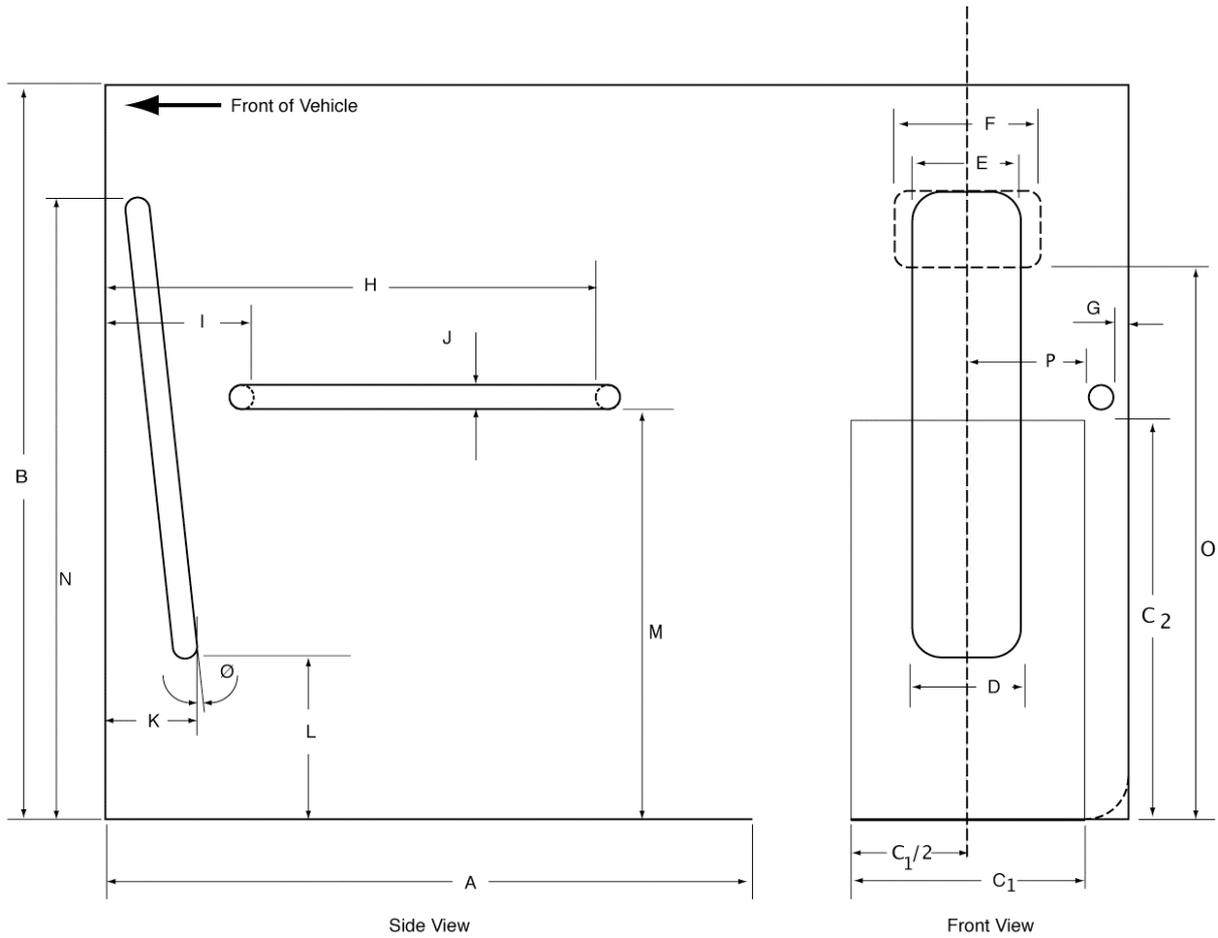
Figure A.1 Specifications for dimensions and clear spaces for a wheelchair passenger space
