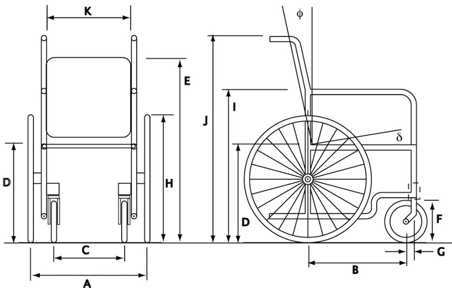
Figure D.1 Critical surrogate manual wheelchair dimensions
