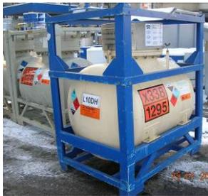
Reusable pressure tanks approved as tank containers or UN portable tanks with a filling capacity in the range of normally 500 to 5000 litres are increasingly being used in the industry, particularly for critical and high-value products. These containers may well be considered as one of the safest types of containment for the transport of dangerous goods.
