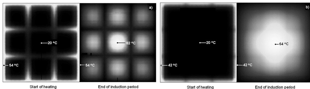
**Fig. 6. Temperature distribution in the stack cross-section .**
