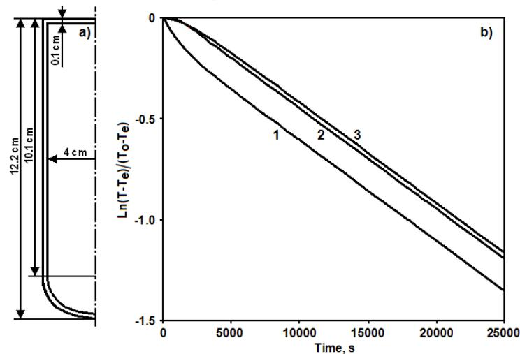
**Fig. 5. Cooling of the Dewar flask.**
