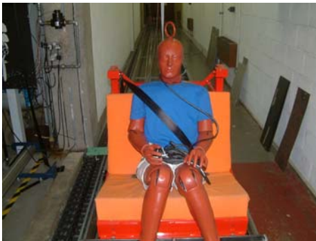
Installation of the Hybrid II dummy on the R44 sled test bench.
