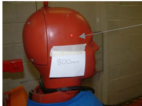
Red Laser point sets to 800mm from Cr. Maximum vertical height from Cr top of 50 th percentile head is 882mm
