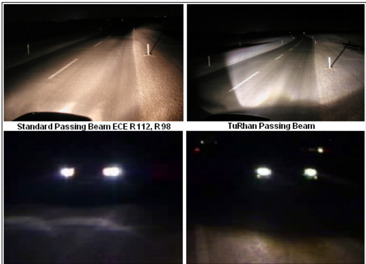
Figure 10: A comparison between standard passing beam and our proposed system for distances and opposing glare effects.
