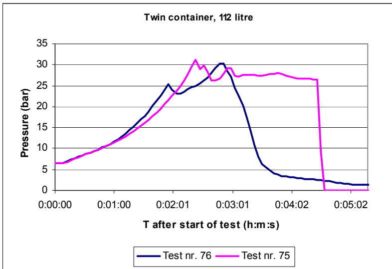
Figure 0.10 Pressure diagrams for two bonfire tests performed on a twin container equipped with the same protection system
