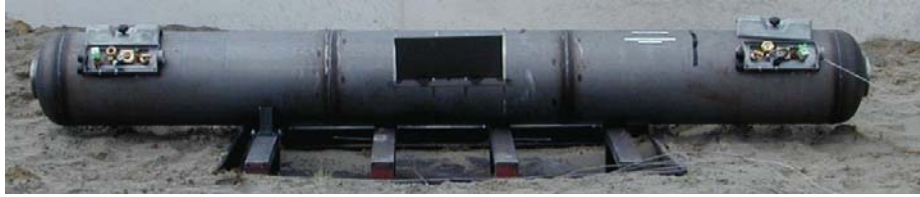
Figure 0.3 Container equipped with a PRV and two fusible plug on three locations
