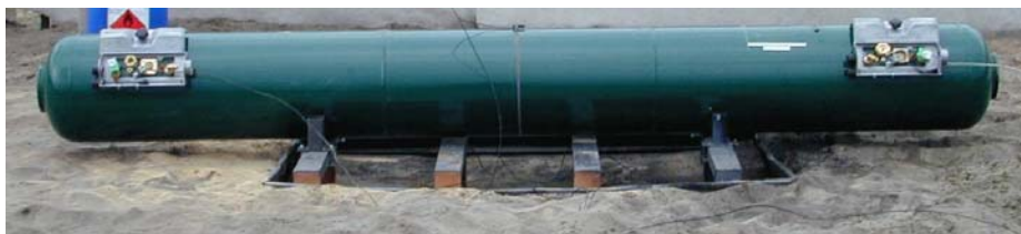
Figure 0.2 Container equipped with a PRV and fusible plug on two locations
