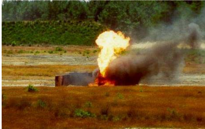
Figure 0.2 Venting of LPG via the PRV resulting in a jet fire with a length of approximately 5 to 10 meters
