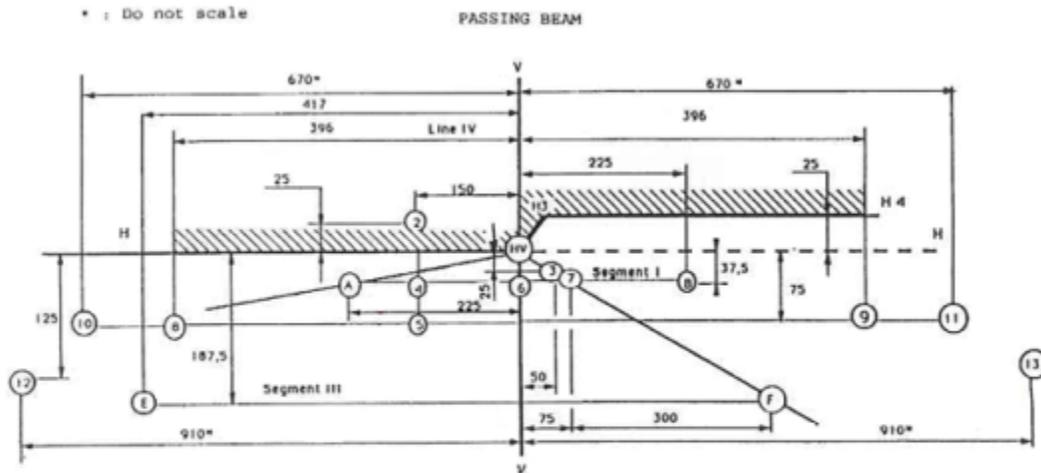
Dimensions are in cm on a flat vertical screen at 25 m. The HH and VV lines are the intersections with this screen of the horizontal and vertical planes passing through the axis of reference of the passing beam as declared by the applicant. The above screen describes a right-hand traffic passing beam. The screen for left-hand traffic passing beam is mirrored about the VV line. Angle HVH2-HH = 15°.
