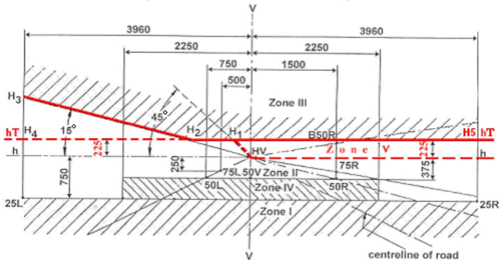
hT-hT : horizontal plane, passes through the focal point of the headlamp
