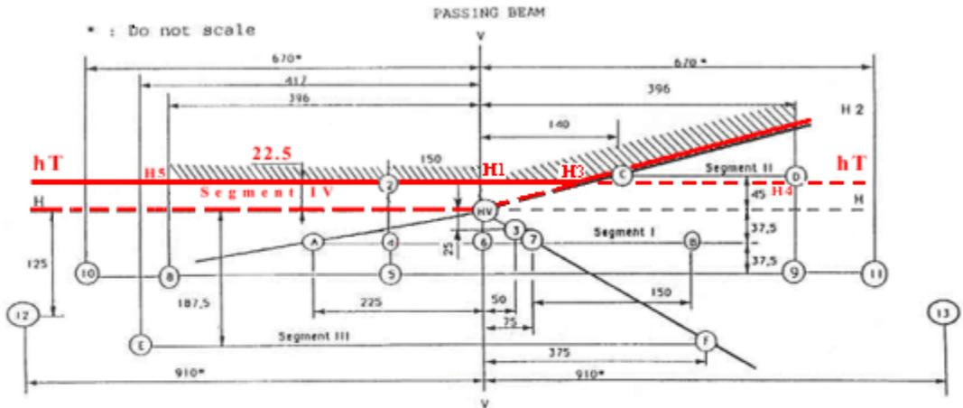
Dimensions are in cm on a flat vertical screen at 25 m. The HH and VV lines are the intersections with this screen of the horizontal and vertical planes passing through the axis of reference of the passing beam as declared by the applicant. The above screen describes a right-hand traffic passing beam. The screen for left-hand traffic passing beam is mirrored about the VV line. Angle H3 H2 - hT hT = 15°
