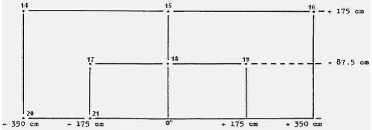
Figure C (Proposed) : Measuring points for illumination values
