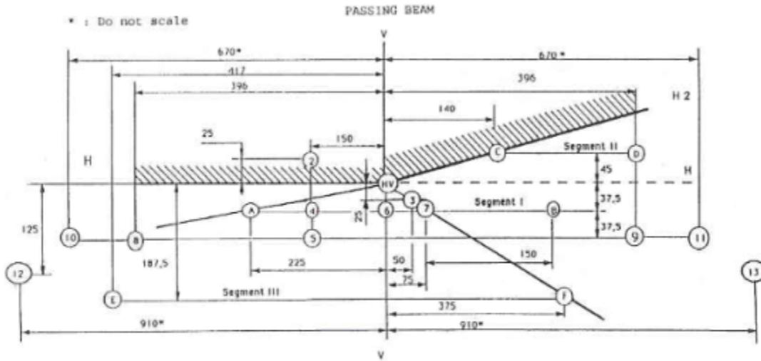
Dimensions are in cm on a flat vertical screen at 25 m. The HH and VV lines are the intersections with this screen of the horizontal and vertical planes passing through the axis of reference of the passing beam as declared by the applicant. The above screen describes a right-hand traffic passing beam. The screen for left-hand traffic passing beam is mirrored about the VV line. Angle HVH2-HH = 15°.
