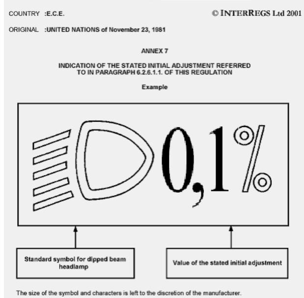
**Annex 7 - Proposed:** In Annex 7 of ECE R48, The “Standard symbol for dipped beam headlamp”, “Value of the stated initial adjustment”, 1.3%, for the unladen vehicle has been changed to 0.1% .
