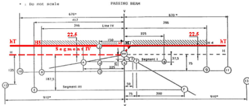
Dimensions are in cm on a flat vertical screen at 25 m. The HH and VV lines are the intersections with this screen of the horizontal and vertical planes passing through the axis of reference of the passing beam as declared by the applicant. The above screen describes a right-hand traffic passing beam. The screen for left-hand traffic passing beam is mirrored about the VV line. Angle H5 H3 - H3 H4 = 0°
