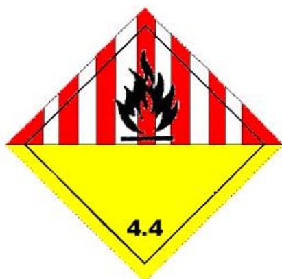
(No. 4.4) Division 4.4 Organic Peroxides Symbol (flame); black Background: upper half: white with seven vertical red stripes; lower half: yellow; Figure: '4.4' in bottom corner
