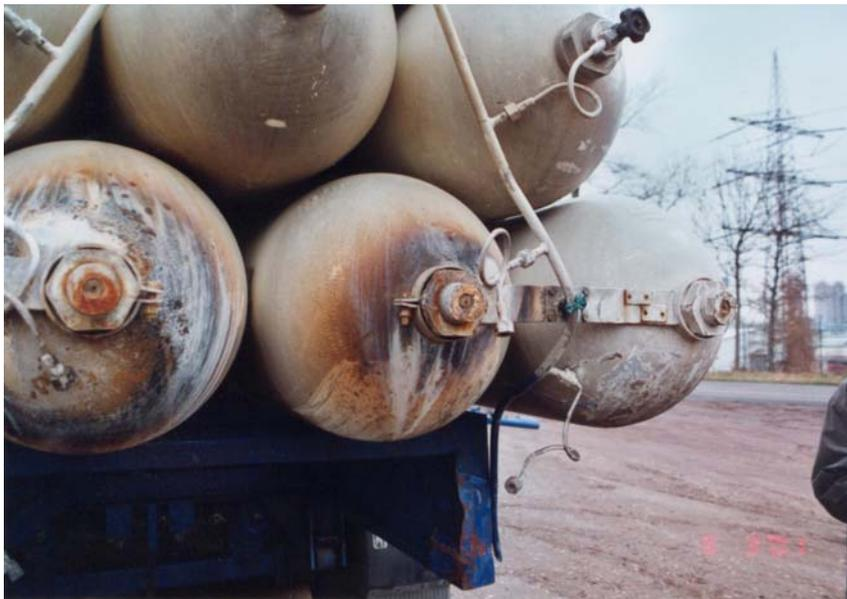
Photo 3: Close-up of the battery vehicle after the accident: first shut-off devices broken off (brass valves), scorch marks caused by hydrogen flames.
