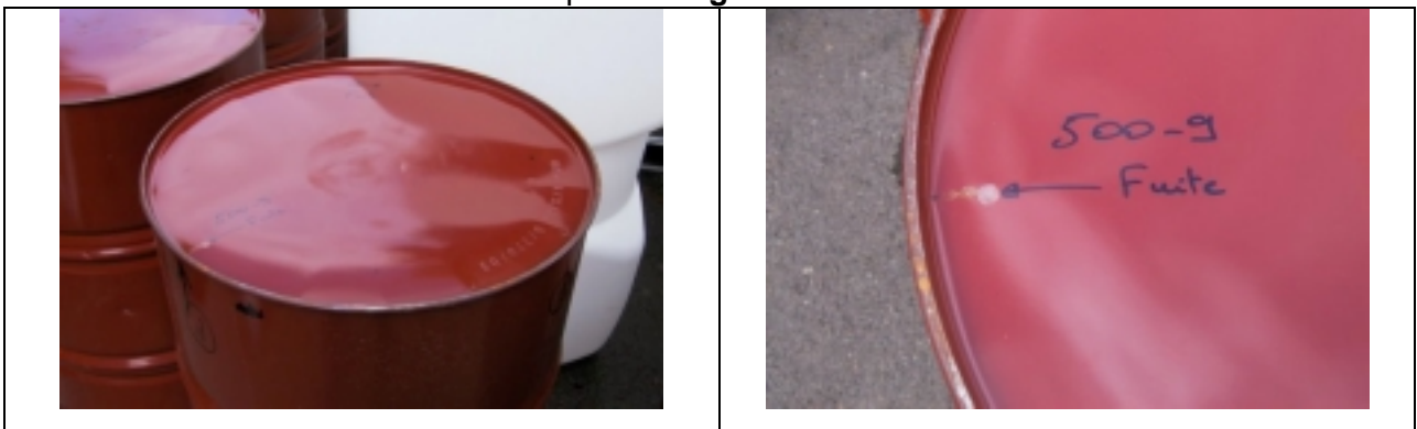
3rd sample: leakage after 48 minutes
