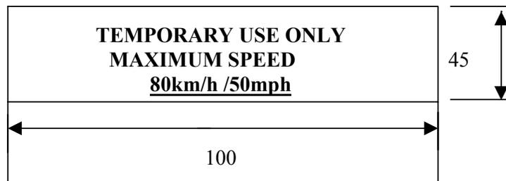
Upper case letters shall be at least 5 mm high and the numbers "80" and "50" shall be at least 20 mm high with the elements that make up each character of the number at least 3 mm line thickness. Lower case text shall be at least have a line height of 5 mm. All text shall be enclosed in a border and be on a background of contrasting colour.
