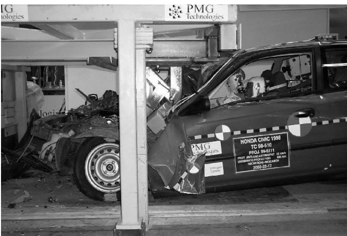
Figure 10. Honda Civic, 480 mm DLG, 56 km/h
