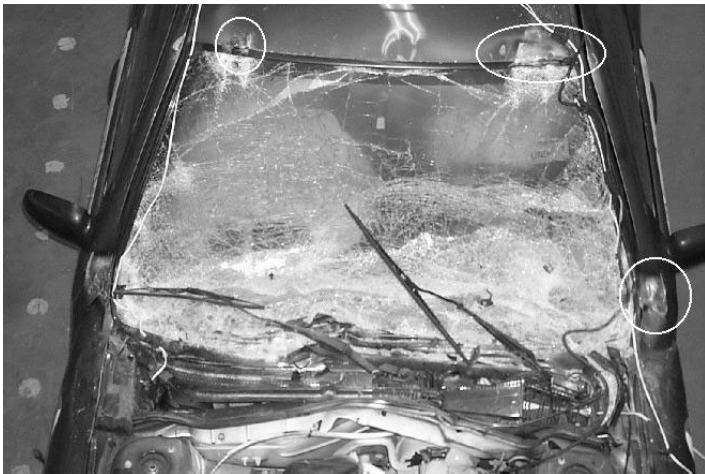
Figure 4. Exterior damage to Chevrolet Cavalier, 560 mm MCG, 48 km/h
