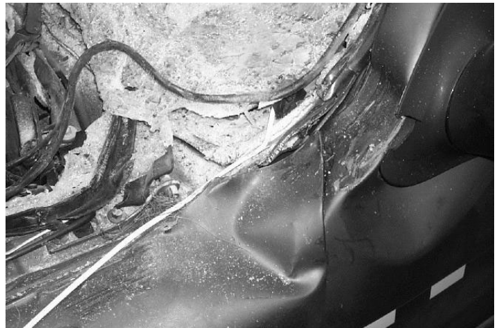
Figure 5. Detail of damage to A-pillar, Chevrolet Cavalier, 560 mm MCG, 48 km/h
