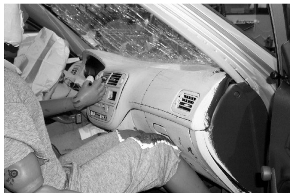
Figure 15. Passenger compartment damage, Honda Civic, Manac Guard, 56 km/h
