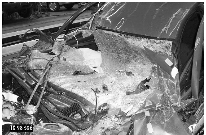
Figure 7. Details of damage to A-Pillar, Chevrolet Cavalier, 480 mm MCG, 65 km/h
