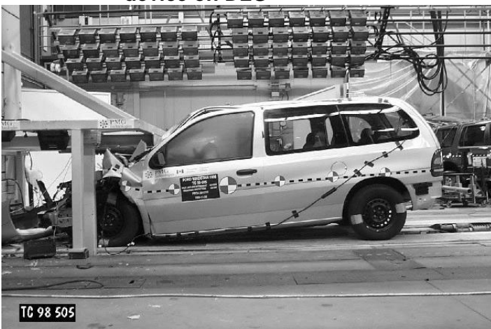
Figure 3. Ford Windstar, 560 mm MCG, 48 km/h
