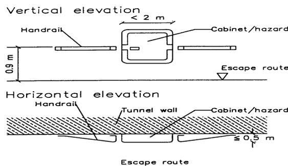
Figure 12.2 Example of guiding system around hazard
