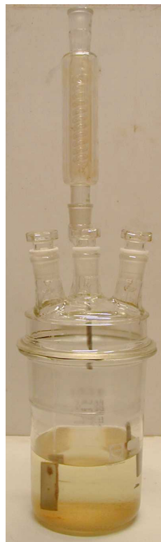
Figure 2: Exposure receptacle with reflux condenser
