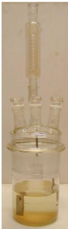
In order to carry out the corrosion test, corrosive medium shall have a minimum volume of 1,5 l to ensure enough reactive agent during the whole exposure time. This is even more important if the corrosion is not caused by the material to be tested but by its quantitatively small amount of impurities.
