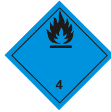
(No. 4.3) Division 4.3 Substances which, in contact with water, emit flammable gases Symbol (flame): black or white; Background: blue; Figure '4' in bottom corner
