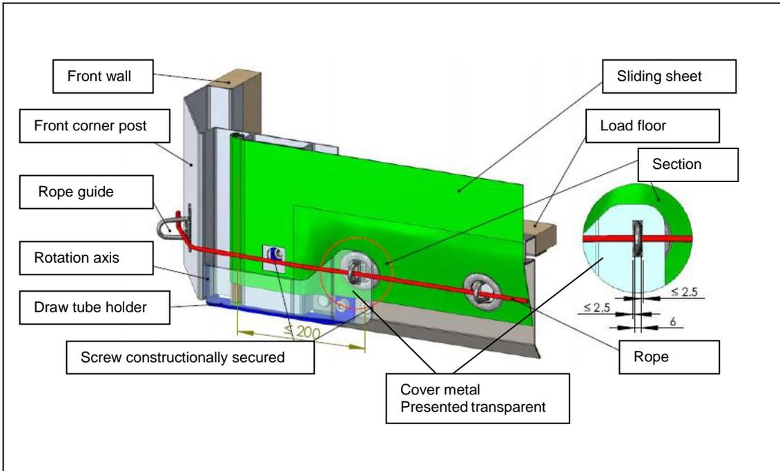
**b) Narrow oval eyelet, anti lifting system for the tensioning tube**
