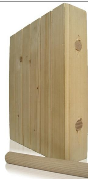
**Notes:** "Brettstapel" board; the plies are held together through long kiln-dried plugs made of beech which are inserted into pre-drilled holes; as soon as they absorb the moisture from the environment they swell leading to a strong bond between the different wooden parts of the board.
