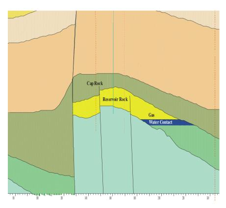
Higher reservoir pressure than hydrostatic in the porous UGS bring higher storage capacity and higher performance of the gas delivery
