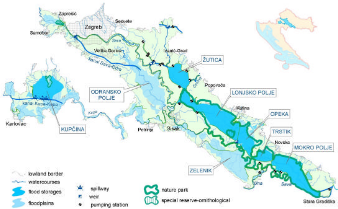
Fig. 5: The Central Sava flood protection system
