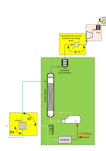
$Q_{stripper} = Q_{sensible} + Q_{desorp} + Q_{water\ vapor}$
