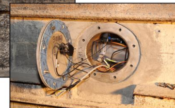
Measurement system – pressure and fire sensors
