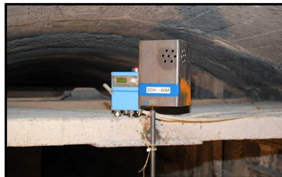
Measurement system – methane sensor
